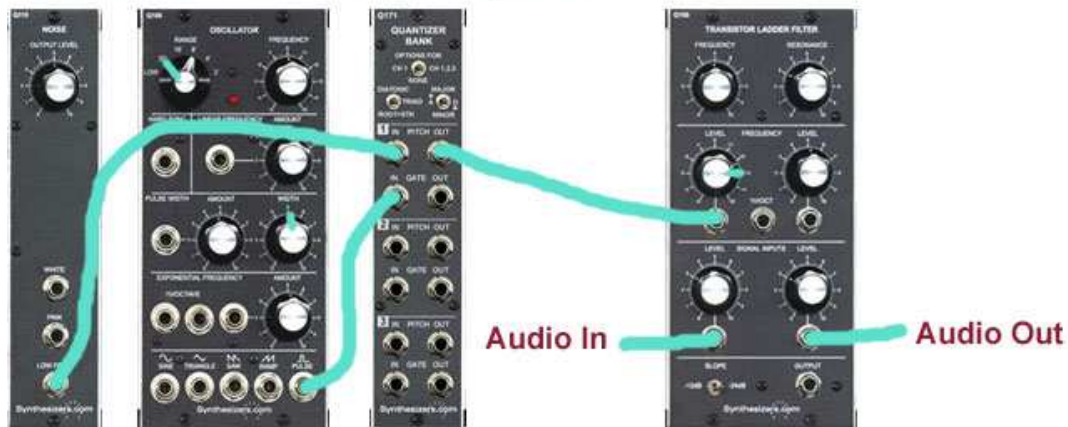
Q171 Quantizer Used as a Sample & Hold
