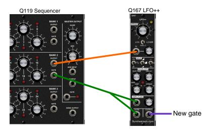
Select square wave, and set the LFO speed so a sequencer knob can produce 1,2,3 or 4 gates per step.
