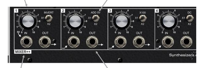
Signal Input for each channel. If no plug is inserted, the signal comes from the input jack of the previous channel. Inserting a plug breaks the chain.
