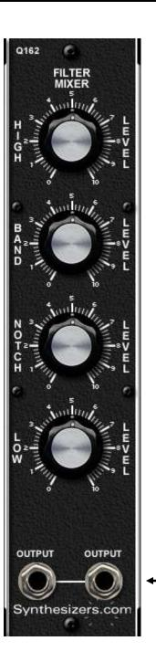
Two outputs available along with individual outputs on the Q107 Filter
