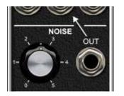
The knob controls a lowpass filter by default but can be changed to control noise level if desired.
