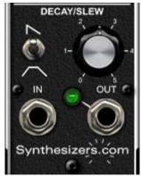
In the slew mode, without a plug inserted, the circuit loops automatically like an LFO to provide gates or modulation signals.
