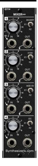
The Q114 Mixer++ has 4 channels with each channel connected to the one above until plugs are inserted. Each channel has a switch offering 3 different functions. This combination of functions and daisychaining provides an incredible amount of signal processing options.
