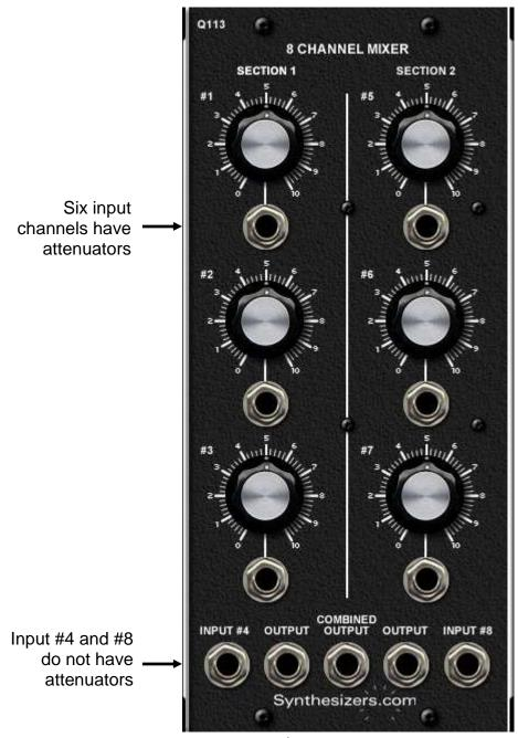
Outputs for each 4-channel section and an output for both sections combined. All available simultaneously.
