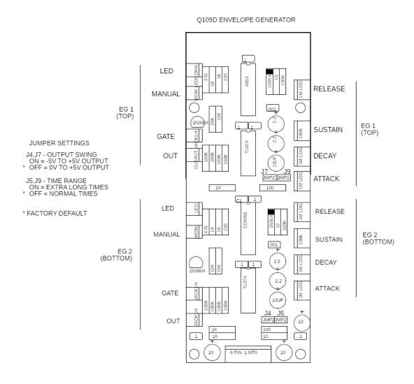
The Q109A-NK Normalization Kit allows for the normalization of the Gate Inputs on the Q109A. A Gate Input in EG 1 will automatically be sent to EG 2 unless a plug is inserted in the EG 2 Gate Input. When a plug is inserted in the EG 2 Gate Input the two sections operate independently.
