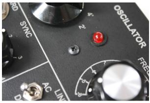
Knobs are removed and attached using a flathead screwdriver on the knob's set-screw.
