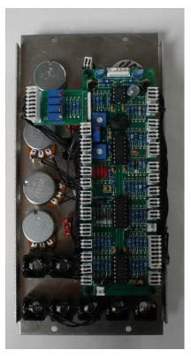
Remove the 3 screws holding in the circuit board, then remove the LED by prying off the ring on the back, then pushing the LED in and removing the bezel.
