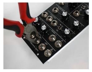
Transfer the components to the new panel. Their location is obvious from the panel graphics. Attach the component's wires to the circuit board using the drawing to match up signals. Then mount the circuit board to the panel with the 3 screws.
